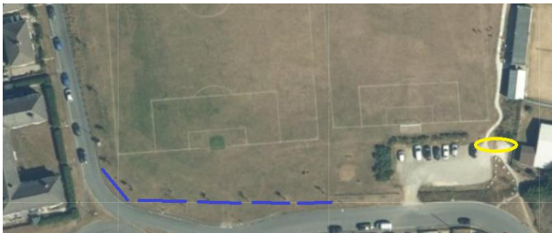
The blue line at the south of the field represents a single rail of key clamps with gaps every 3m for pedestrian access.
